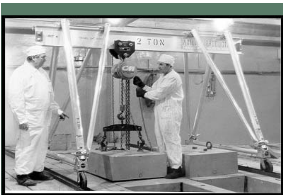
HISTORICAL ACHIEVEMENT: Material protection upgrades at a Russian nuclear facility increase security by delaying access to stored nuclear materials. Stored plutonium is secured under one ton concrete blocks requiring a two-person crane to move. See pages 4 and 5 for more about NNSA's achievements in the largest U.S.-Russian cooperative threat reduction effort in history.
